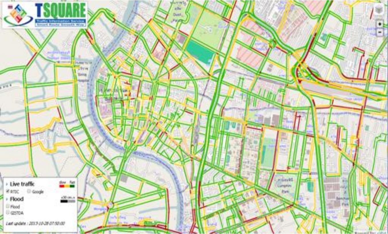
GPS data from taxis (Taxi Probe Data) can monitor traffic condition of detailed streets.
